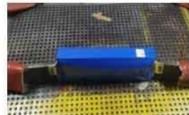
Fig. 7 Short circuit test photo for 014
